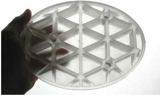
**Figure 13. The light-weight cast borosilicate secondary mirror made by Optical Structures.**
